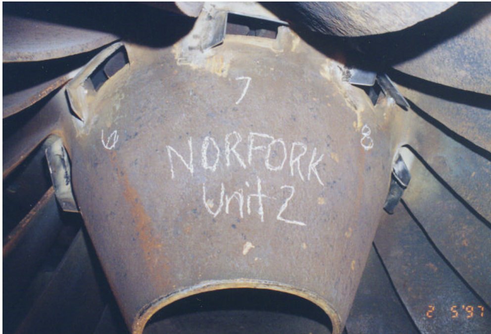
Figure 5. Hub Baffles Installed at Norfolk Dam
